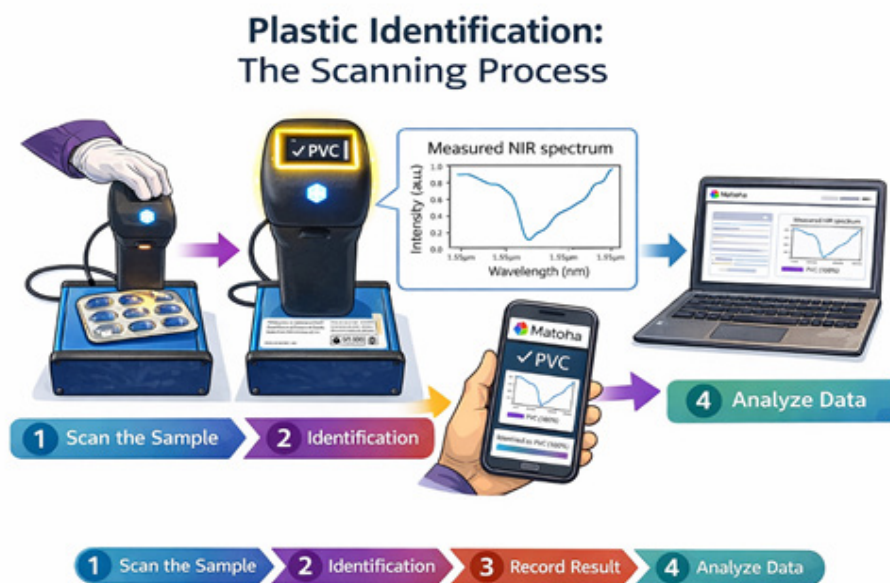
Fig. 3. Schematic representation of the material identification workflow using handheld NIR spectroscopy.
