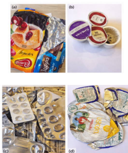
Fig. 1. Representative aluminium–polymer composite packaging waste samples: (a) flexible food packaging; (b) coffee/tea capsules; (c) pharmaceutical blister packs; (d) dairy packaging lids.
