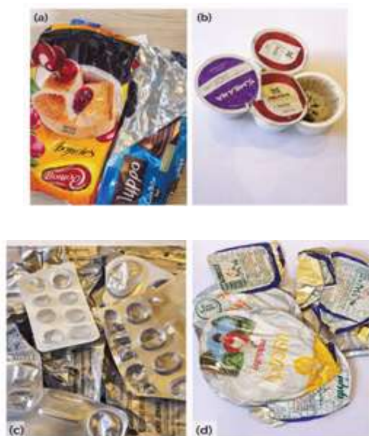
Fig. 1. Representative aluminium–polymer composite packaging waste samples: (a) flexible food packaging; (b) coffee/tea capsules; (c) pharmaceutical blister packs; (d) dairy packaging lids.
