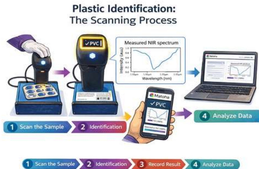
Fig. 3. Schematic representation of the material identification workflow using handheld NIR spectroscopy.
